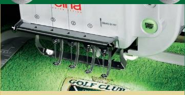
Totally autonomous operation! Automatic colour change, thanks to four separate needles.
