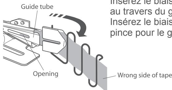
Pull 2" (5 cm) of the tape out of the muzzle of the tube, and fold the tape at a right angle.
