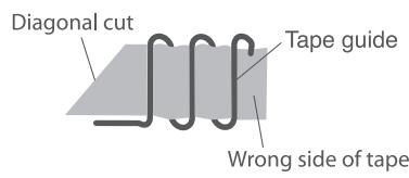
Insert the tape with its wrong side facing you, through the tape guide back and forth.
