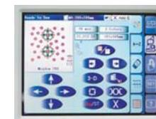
Move the hoop until the needle passes through the Exact Center of the "Starting Point" hole in the template.
