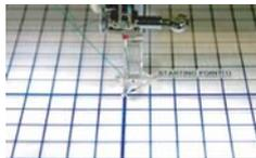
Detach the hoop from the machine and shift the frame to position 2 and reattach to machine.
